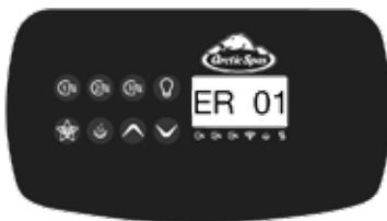
ER01 – Flow Switch
